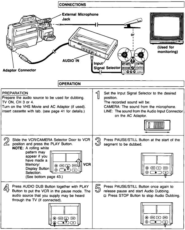
**NOTE:** When a microphone is used for dubbing, do not place it near the speaker of your TV while dubbing is being done. A howling noise (feedback) may occur.
