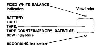
Check the EVF display to confirm conditions of battery, lighting, and other functions.
